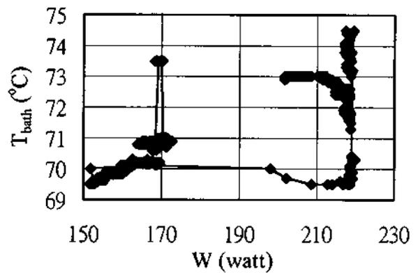
Fig. 6. The plot of  $T_{bath}-W$  for a Ni/Pt/ $H_2O/K_2CO_3$  cell
