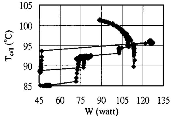
Fig. 10. The plot of  $T_{cell}-W$  for a Pd/Pt/ $D_2O/LiOD$  cell
