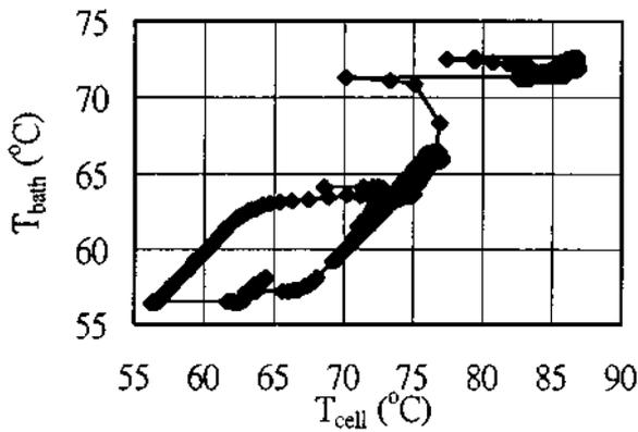
Fig. 5. The plot of  $T_{bath}-T_{cell}$  for a Ni/Pt/ $H_2O/K_2CO_3$  cell
