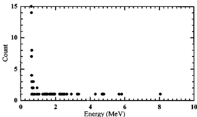
Figure 4 Si-SSD spectrum (Exp.1-33, Live time 3,580sec)
