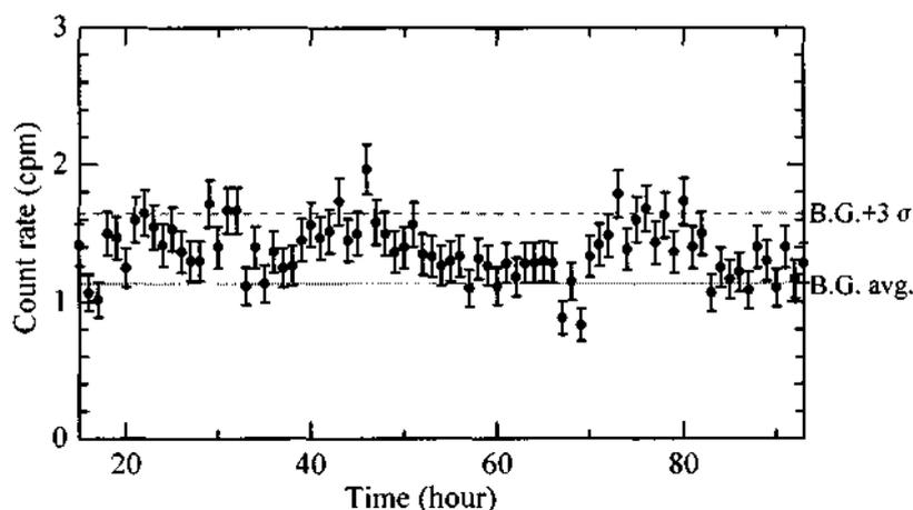
Figure 5 Neutron measurement in the gas loading experiment with Pd plate sample (Exp. 2-02)
