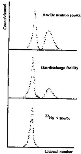
Fig 2. n- $\gamma$  discriminating spectra of gas-discharge neutron
