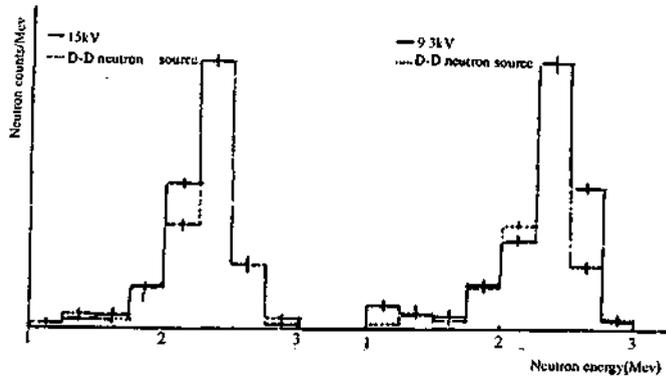
Fig 4. The neutrons spectrum produced by gas-discharge
