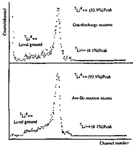
Fig 1. Characteristic spectra of the pulse height distribution for  $^{10}\text{B} (n, \alpha) ^7\text{Li}^{\beta}$  reaction
