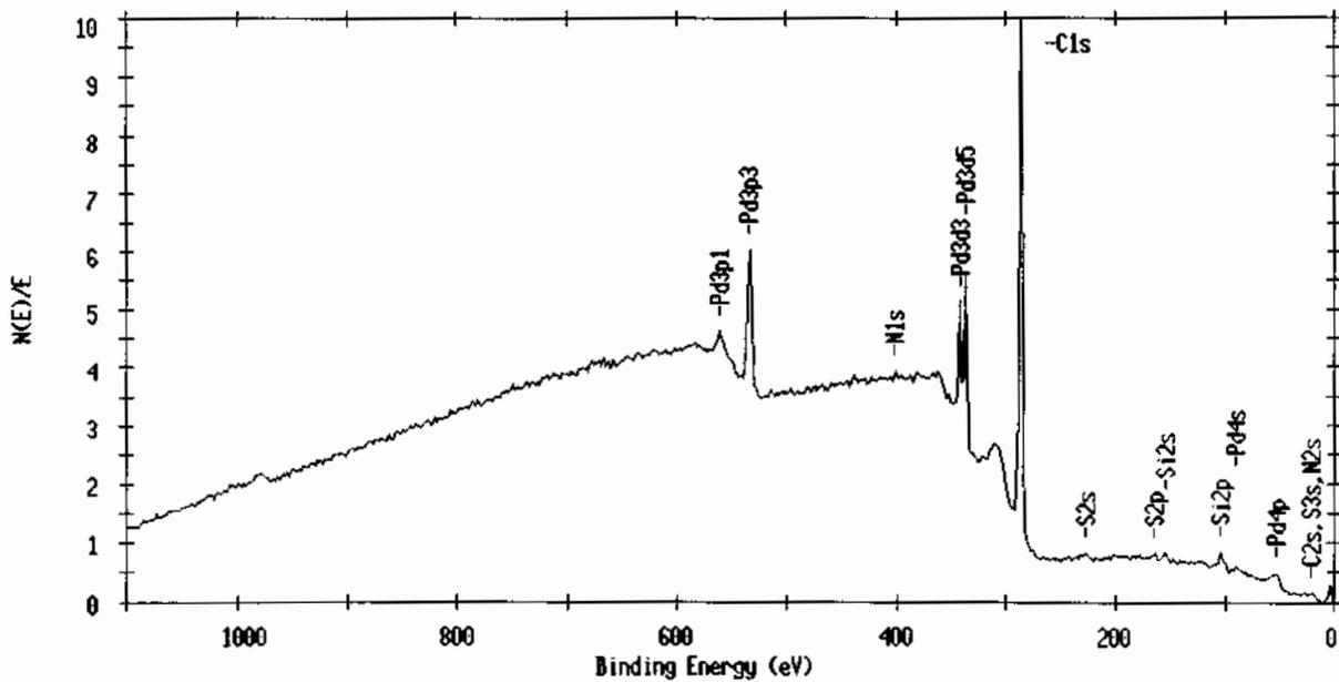
Fig. 5 XPS spectrum of the Pd point electrode after neutron emission
