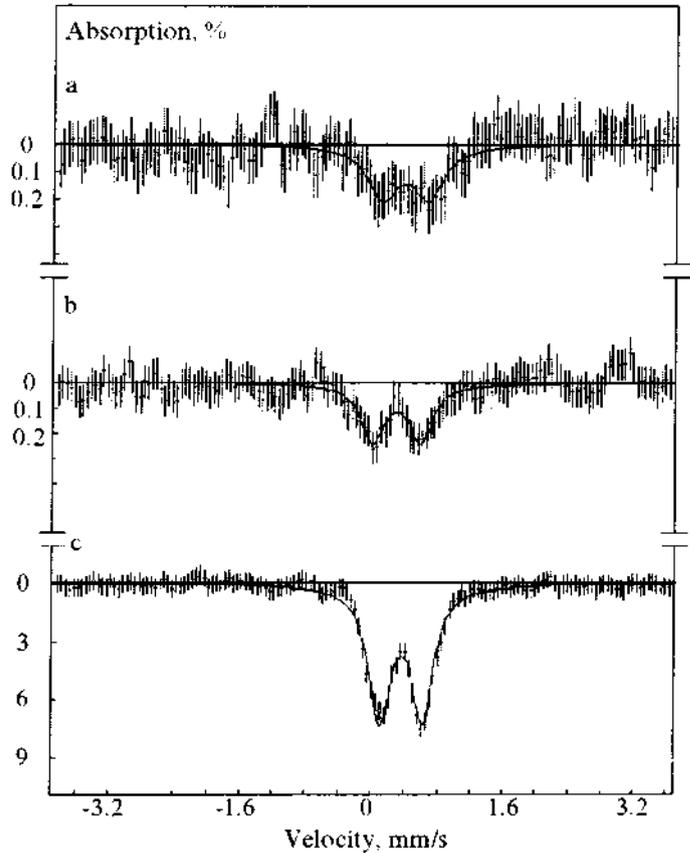
Fig. 3. Mossbauer spectra of grown cultures. Culture *Deinococcus radiodurans* grown: a) and b) in  $\text{D}_2\text{O}$  with present  $\text{Mn}^{55}$ ; c) in  $\text{H}_2\text{O}$  with present  $\text{Mn}^{55}$  and small quantity of  $\text{Fe}^{57}$ .
