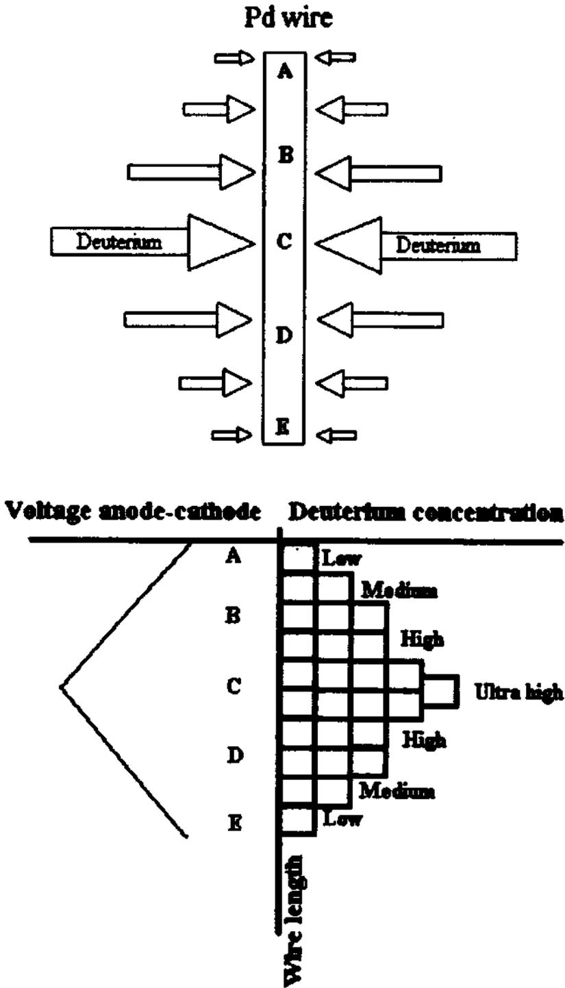
Fig.5: Sketch of enhanced electromigration by "central wire geometry" (collider). The point C is the most negative input voltage, the points A and E are electrically connected.
