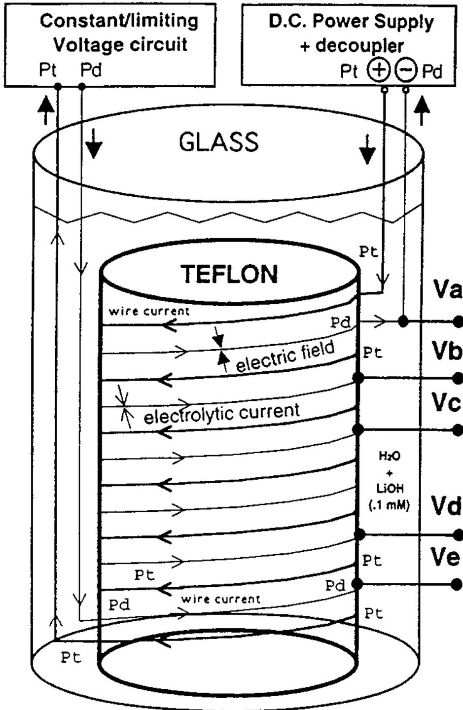
Fig. 1: Electrolytic cell. Pd/Pt double twisted wires on teflon cylinder sample-holder.
