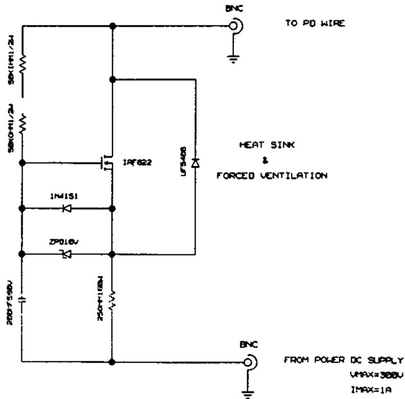
Fig.4: Details of "high impedance booster" electronic circuit.
