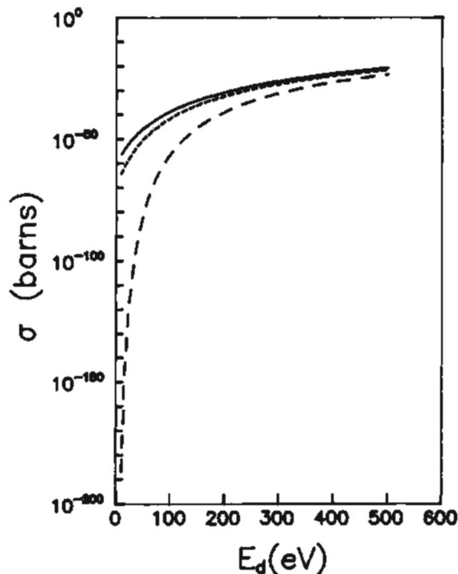
Fig. 2. The deuteron-deuteron calculated fusion cross section as a function of the CM kinetic energy  $E_d$ . In the long dashed curve is the prediction for the  $d + d$  Coulomb repulsive potential, in the solid curve for the  $(D + D)$  potential in  $D_2$  molecule [7], and in the short dashed curve for the partially screened  $d + d$  potential in  $D_2^-$ .
