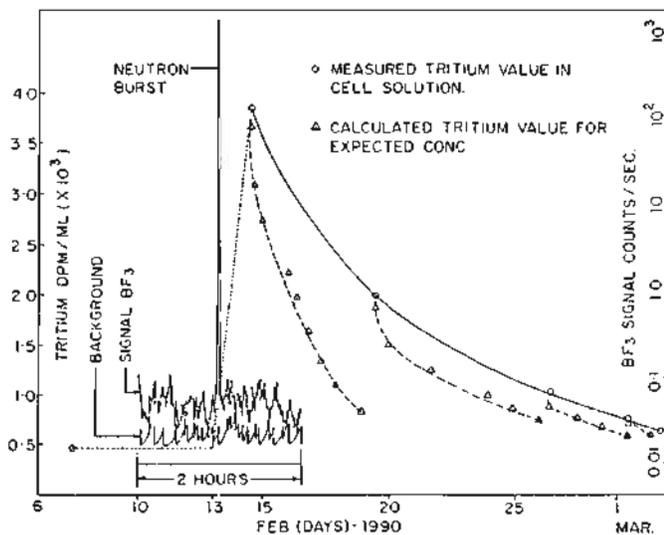
Fig.7. Neutron and Tritium Output of RCS-11 Experiment
