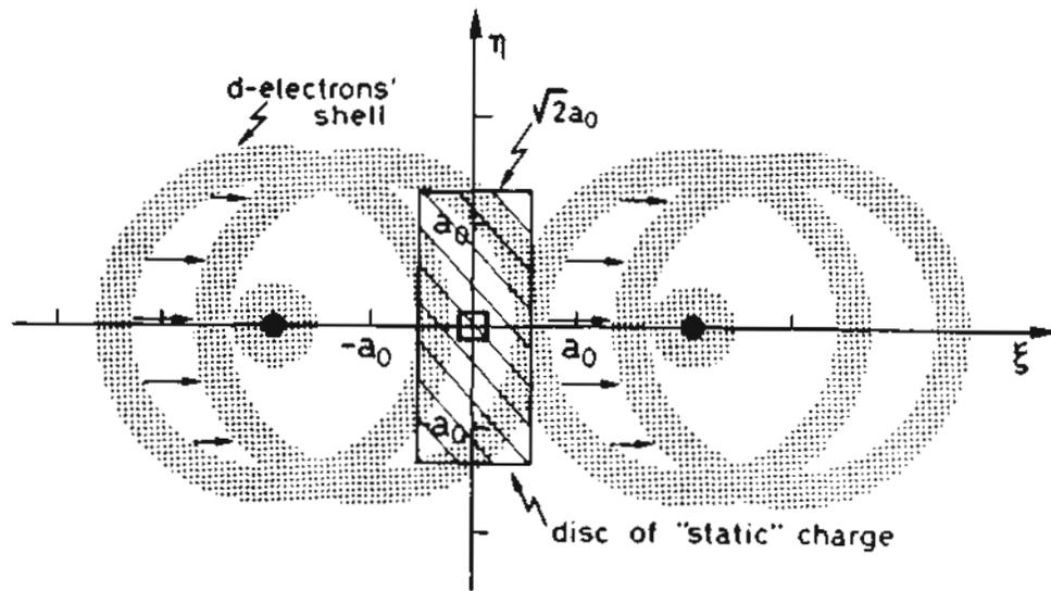
Fig.2 The d-electrons' plasma oscillations between nearest Pd-neighbors.  $a_0$  is the Bohr radius ( $.57\text{\AA}$ )
