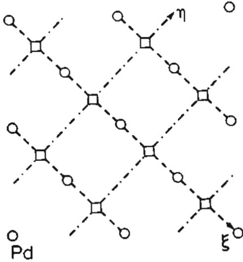
Fig.1 A plane of the Pd-lattice. The sites denoted by a circle are occupied by the Pd-nuclei, while those denoted by a square are occupied by D-nuclei.  $\xi$  and  $\eta$  are the two orthogonal directions linking nearest Pd neighbors. The dashed lines shall be called  $\xi$ -lines, the dash-dotted  $\eta$ -lines.
