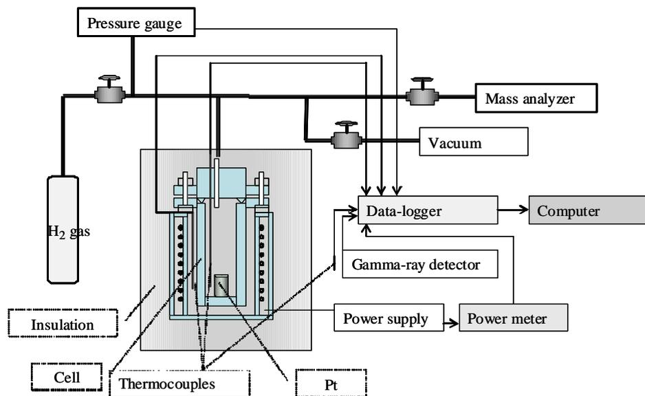
Figure 2. Schematic drawing of the measurement setup.
