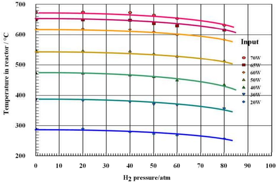
**Figure 5. H<sub>2</sub> pressure dependence of reactor temperature at various input power.**
