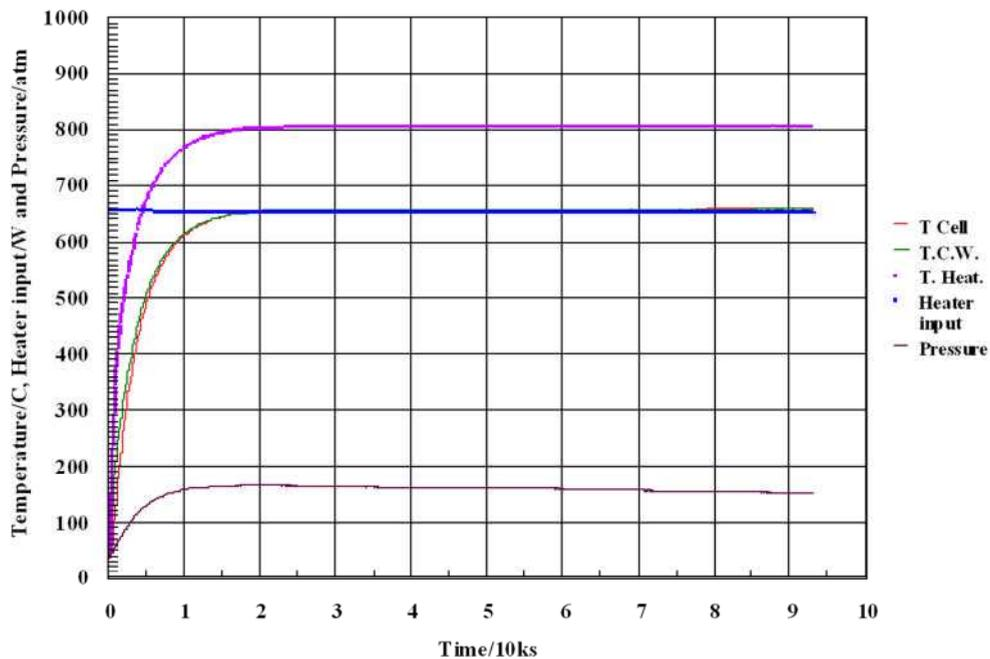
Figure 3. Temperature, pressure and heater power with the Inconel reactor at 650 W input and H<sub>2</sub> at 50 atm with no phenanthrene sample. Three temperatures are measured in this test: inside the cell (T cell) at the cell wall (T.C.W), and at the heater (T. Heat.).
