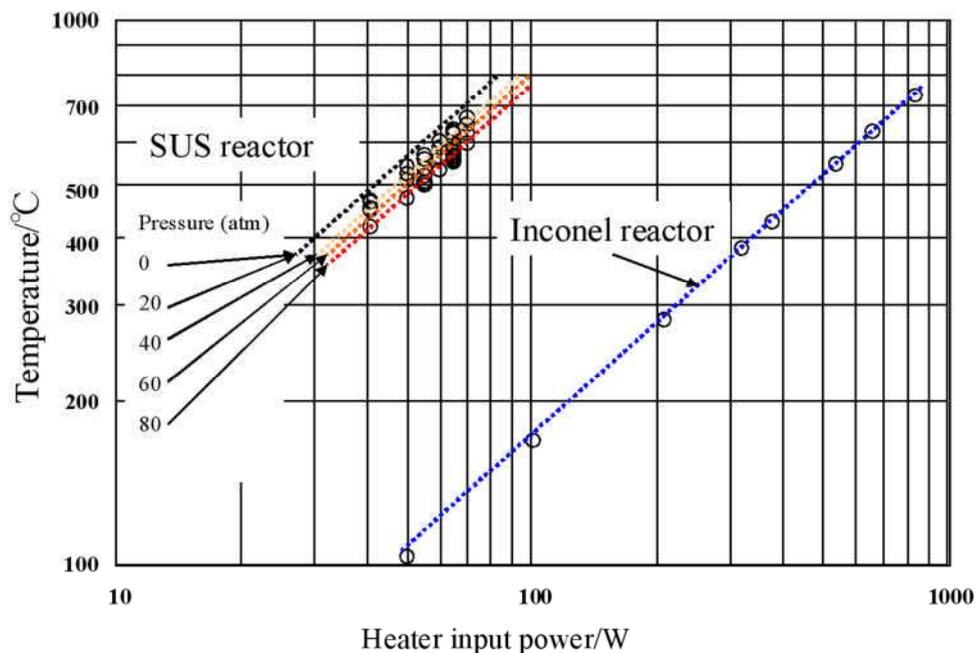
Figure 4. Heater input dependence of reactor temperature at various H<sub>2</sub> pressure settings.
