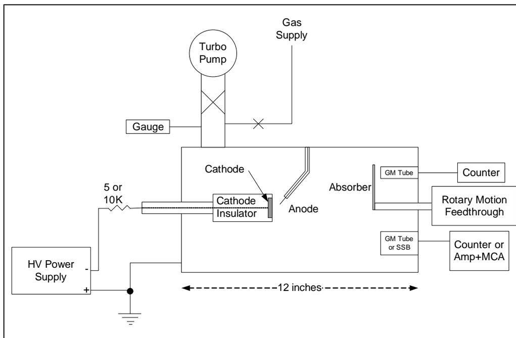
**Figure 1. Diagram of experimental apparatus**
