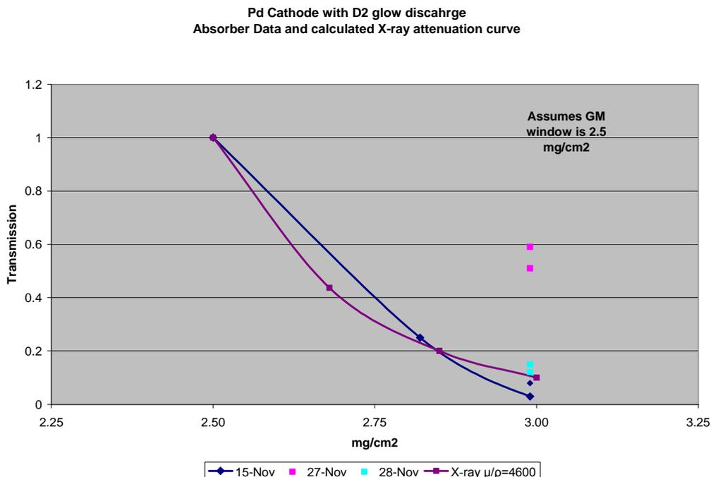
**Figure 12. Attenuation vs. total absorber thickness. X-ray attenuation assumes an attenuation coefficient ( $\mu/\rho$ ) of 4600 cm<sup>2</sup>/gm which is obtained by extrapolating the NIST aluminum curve to 600 eV.**
