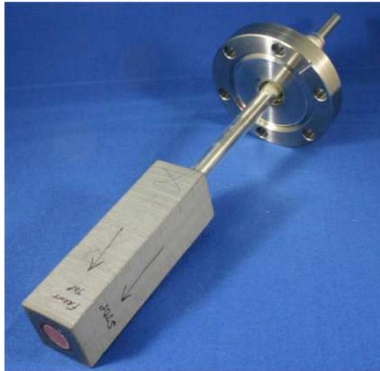
**Figure 3. Cathode insulator assembly**
