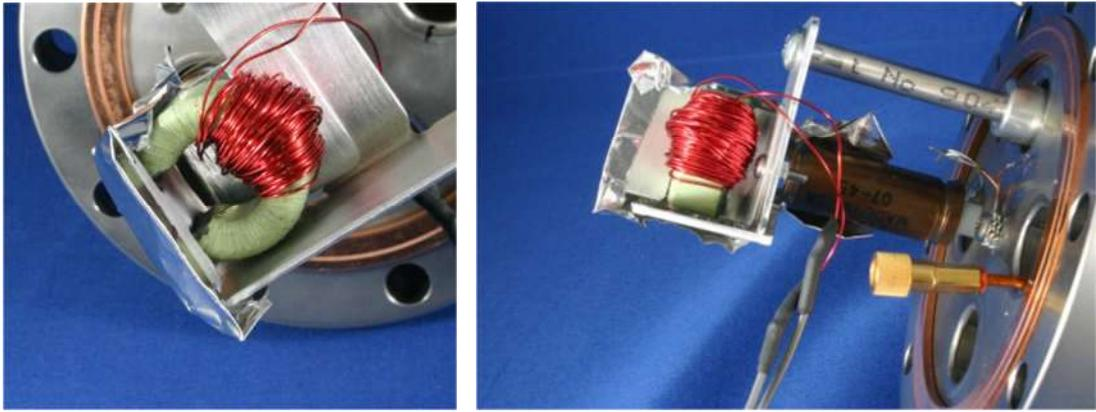
Figure 7. Photographs of deflection assembly using electromagnet with slit in front GM tube
