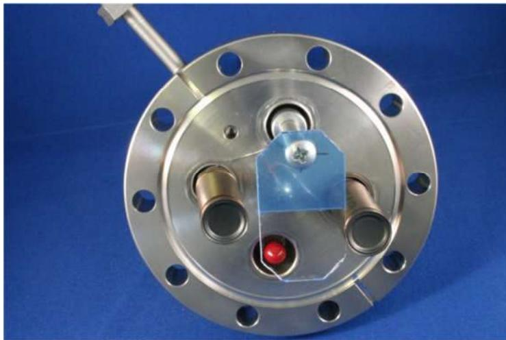
**Figure 4. Detector end-plate configured with dual GM tubes and plastic absorber. (CR-39 is used here as a  $100\text{mg}/\text{cm}^2$  absorber.)**
