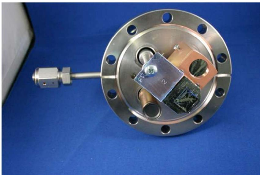
**Figure 5. Detector end-plate configured with  $2\text{mg}/\text{cm}^2$  GM tube, Si detector, 1.8 micron aluminum absorber and CR-39 detector.**
