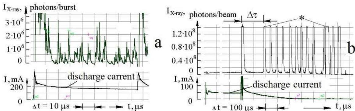
Figure 3. The typical oscillograms of the X-ray emission signal from the system scintillator – PM. The cathode sample is Pd, D<sub>2</sub> discharge. a – diffusion mode, b – form of laser beams; \* - the pulse peak was cut a discriminator of amplifier.
