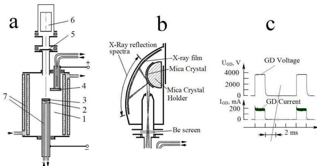
**Figure 1.** Schematic representation of the experiment. a. Glow discharge device, 1 – discharge chamber, 2 – cathode holder, 3 – cathode sample, 4 – anode, 5 – Be foil screens, 6 – X-ray detectors different kind (pinhole, TLD detectors, scintillator- photomultiplier, spectrometer), objective, 7 –cooling water; b. X-ray spectrometer, c. Glow discharge voltage and current oscillograms.
