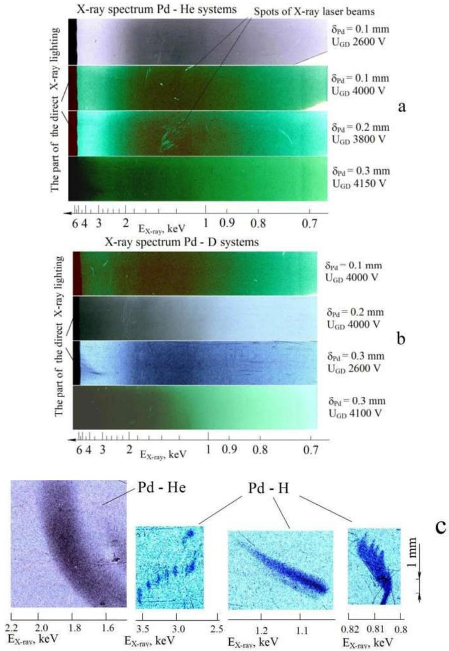
Figure 5. X-ray energy spectra. a, b – during the glow discharge operation, c – after the glow discharge in the spot modes.
