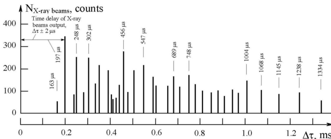
Figure 4. Temporal characteristic of X-ray beam emissions. The cathode sample is Pd, D<sub>2</sub> discharge, current 50 mA.
