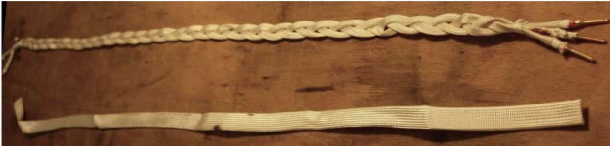
**Figure 2. Three wires braided together: 1 coated Pd wire and 2 Pt wires (Pt<sub>cal</sub>, Pt<sub>mon</sub>). Each wire is 50 μm in diameter. The diameter of the fibre-glass sheaths is 2 mm. The braid is completely covered inside a larger sheath (6 mm) shown below. Ultra-pure (>99.99%) Pt was used for Pt<sub>cal</sub> and Pt<sub>mon</sub>. Pt<sub>cal</sub> serves as a calibration Joule heater and Pt<sub>mon</sub> serves as a distributed thermometer.**
