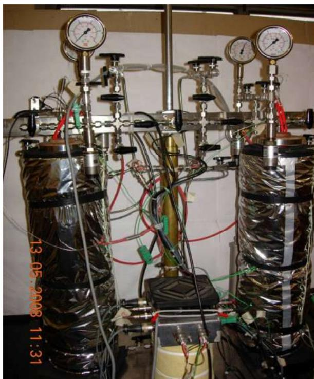
**Figure 1.** The twin chamber differential reactor developed at INFN-LNF. Pressure: up to 100 bar. Temperature: up to 320°C. Useful volume of the crucibles: 15 cm<sup>3</sup>.
