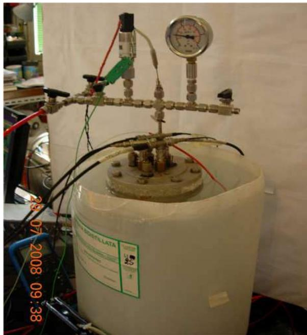
**Figure 4. The pressurized experimental cell surrounded by a large water bath.**
