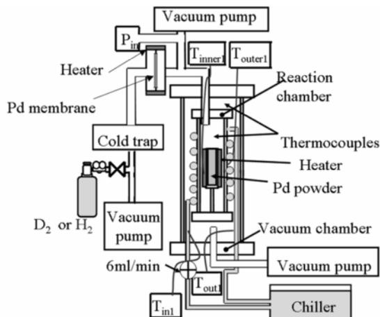
Figure 2. Functional view of the system
