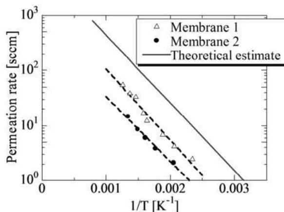
Figure 4. Permeation characteristics of the Pd membrane filter.
