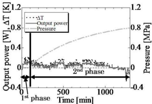
Figure 7. Absorption run for the 0.1- $\mu\text{m}$ -diam. Pd powder. The  $\text{D}_2$  gas flux is 3.5 sccm.
