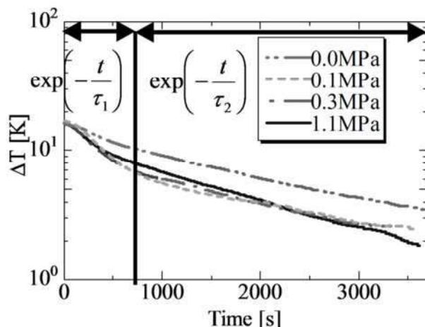
Figure 3. Calibration of flow calorimetry
