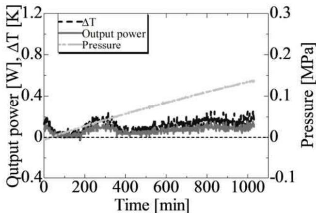
Figure 5. Evolution of temperature, heat and pressure in the vessel after exposure of the 150 mesh Si powder to D<sub>2</sub> gas.
