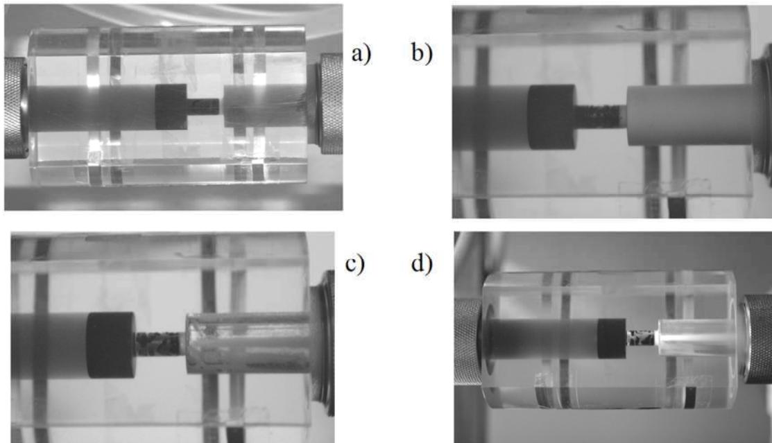
**Figure 2. General view of the working chamber: a) at low pressure ( $P < 20$  atm) of moving oil; b) at the beginning of the cavitation process ( $P = 25 \dots 40$  atm); c) at separation of the liquid stream from the chamber walls at the condition of intensive cavitation ( $P > 60$  atm). d) Bright luminescence of the directed liquid stream with cavitation bubbles ( $P \geq 80 \dots 90$  atm).**
