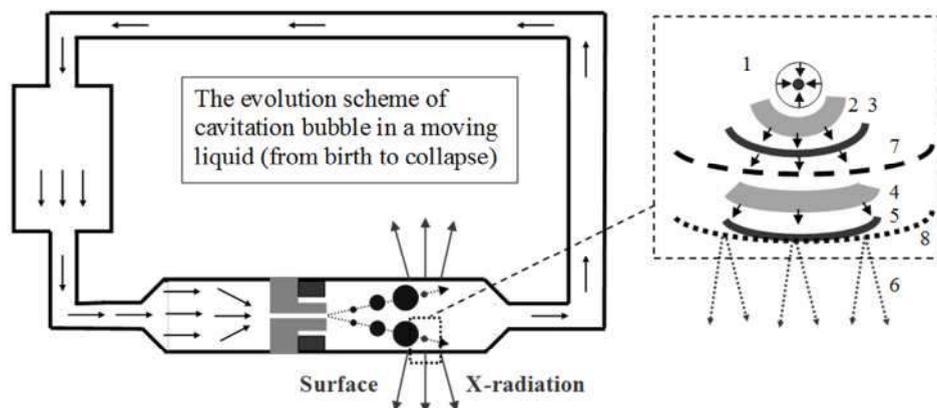
**Figure 7. Schematic of transformation of the energy of bubble cavitation collapse to the outside X-ray radiation: 1) - cavitation collapse; 2) acoustic impulse; 3) shock wave in liquid; 4) formation of elastic wave in the wall of the cavitation chamber; 5) shock wave in the wall of the cavitation chamber; 6) excitation of surface atoms of the cavitation chamber during the reflection of shock wave; 7) and 8) internal and external surfaces of the cavitation chamber wall.**
