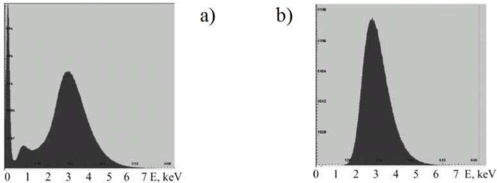
**Figure 4. Spectrum of X-Ray radiation outside of the chamber during cavitation in the presence of: a) copper powder, mechanically and acoustically connected with its external surface; b) the same powder and additional thin copper absorber which has not been mechanically connected with the chamber.**
