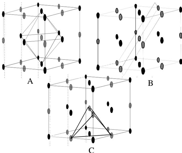
**Figure 3. In Lower Concentrations, Hydrogen is in Sites with Octahedral Symmetry in an fcc Lattice. An Octahedron Enveloping a Hydrogen Nucleus is Seen on the Left. A Plane Square Sub-Lattice Containing the Octahedral Hydrogen Nuclei is Indicated on the Right. A Tetrahedron with a Hydrogen Nucleus on Each Vertex is Shown Below.**
