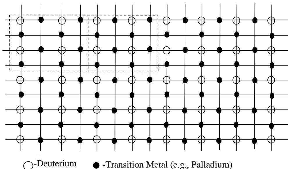
**Figure 1. Two-Dimensional Arrangement of Transition Metal and Deuterium in a Disposition Similar to That in the Active Planes of Typical High-Temperature Superconductors.**
