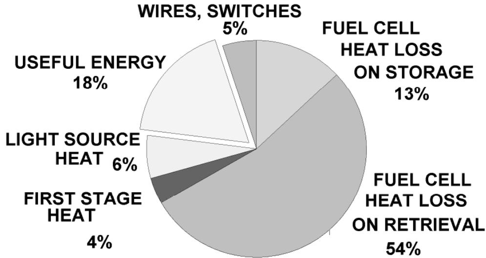
**Figure 2 - Losses in the Feedback Loop of the JET Energy Self-sustaining LANR Electricity System**
