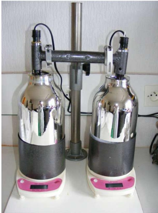
**Figure 6. Differential calorimeter**
