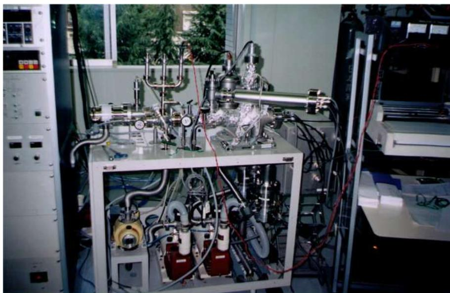
Figure 5. Stainless steel (ss) manifold system used in analysis of desorbed gases
