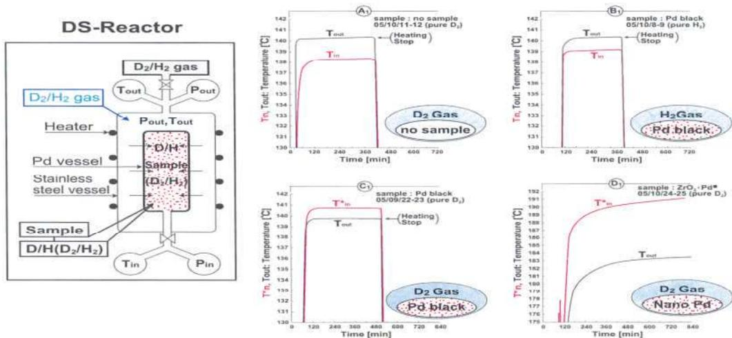
Figure 10. Gas loading tests at elevated temperature
