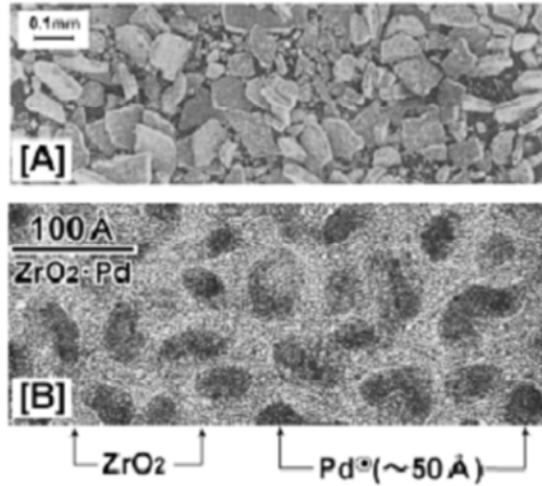
Figure 7. New catalyst shows nano-Pd embedded in ZrO<sub>2</sub>
