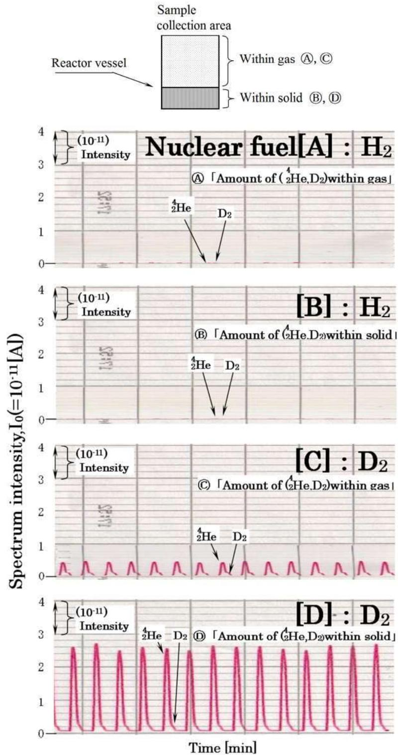
Figure 7. Mass analysis result for fuel (H<sub>2</sub> or D<sub>2</sub>) and reaction product (<sup>4</sup>He)
