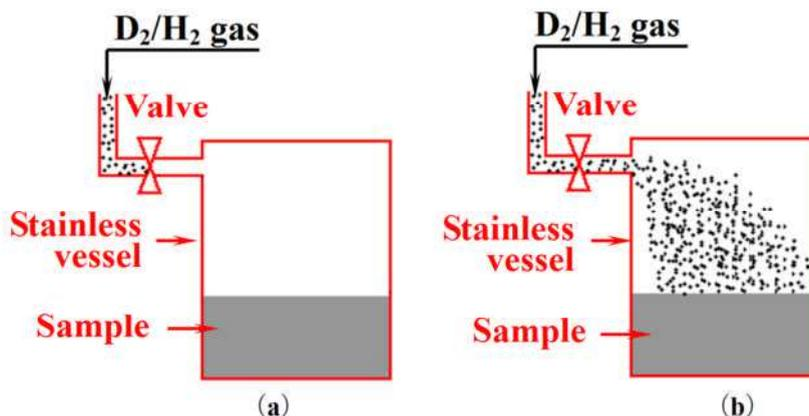
**Figure A. Principle of "Solid Fusion" Reactor Vessel. (a): Reactor before introduction of D<sub>2</sub> or H<sub>2</sub> gas (only stainless steel vessel and sample (b): Introducing of D<sub>2</sub> or H<sub>2</sub> as the D<sub>2</sub> or H<sub>2</sub> "jet-stream" into reactor vessel; and then D<sup>+</sup> or H<sup>+</sup> "jet stream" penetrate into the sample)**
