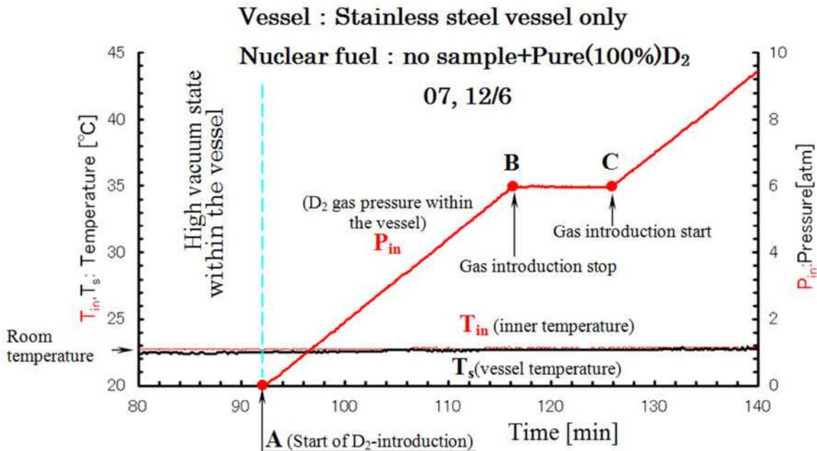
**Figure 6. Gas pressure characteristics within vessel (no sample)**
