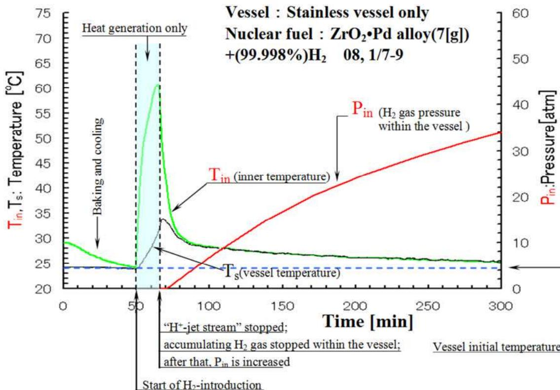
**Figure 4. Heat Generation for H<sub>2</sub> Introduction**
