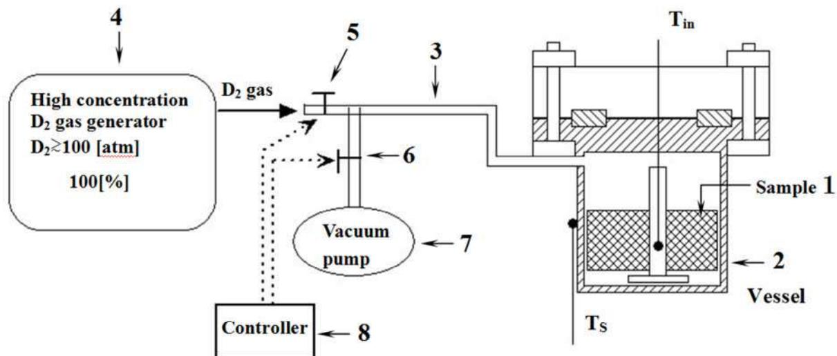
Figure 1. Experimental Device
