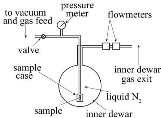
Fig. 2 - Scheme of the experimental set-up.
