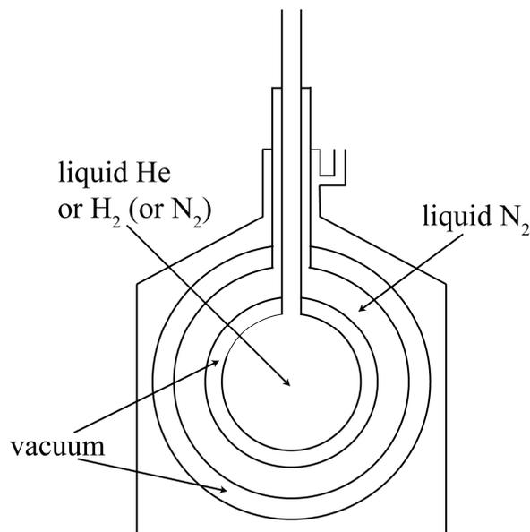
Fig. 1 - Schematic drawing of a Supairco “old style” liquid He/H<sub>2</sub> dewar.
