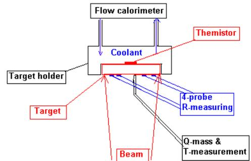
Fig. 3 - Target holders with water cooling.
