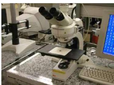
Fig. 5 - System for tracks count
