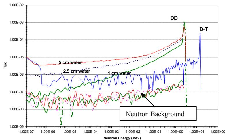
Fig. 3. - Calculated neutron spectra as a function of the Radius R at the detector's position
