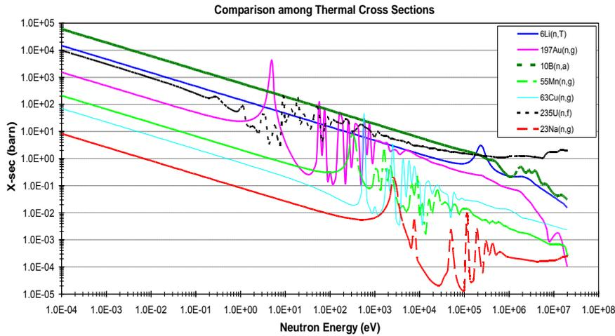
**Fig. 1.** - Cross-section versus neutron energy for some materials.
