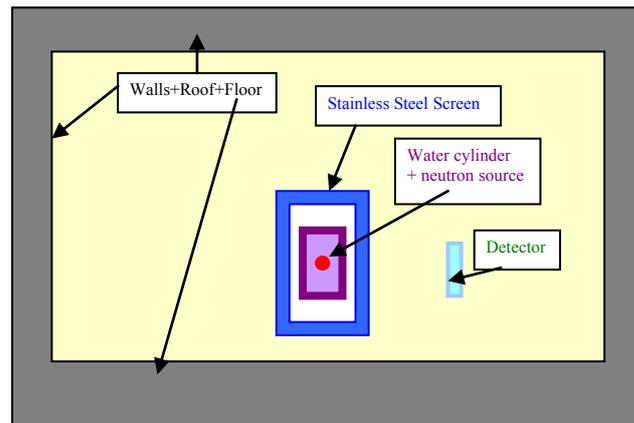
Fig. 2. - MCNP Model of a CMNS experiment
