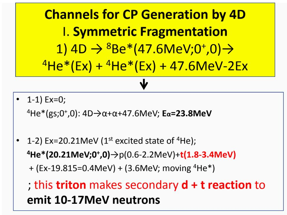
Fig.1 - Generation of tritium by a symmetric fragmentation of <sup>8</sup>Be\* by 4D fusion and its secondary t + d reaction to emit high energy neutrons in a 10 – 17 MeV region which may correspond to the SPARWAR result.
