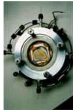
Fig.3 - MIII, 46 KHz reactor, had two opposing piezos with a calibration heater.
