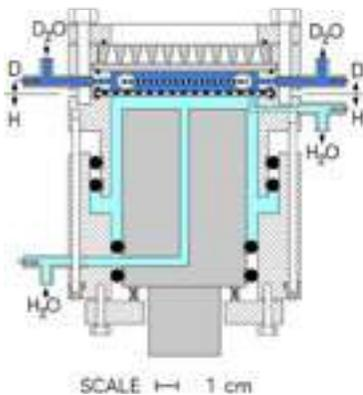
Fig.1- MII, reactor 20 KHz was used in the tritium and  $^3He$  experiment with a heater for calibration.
