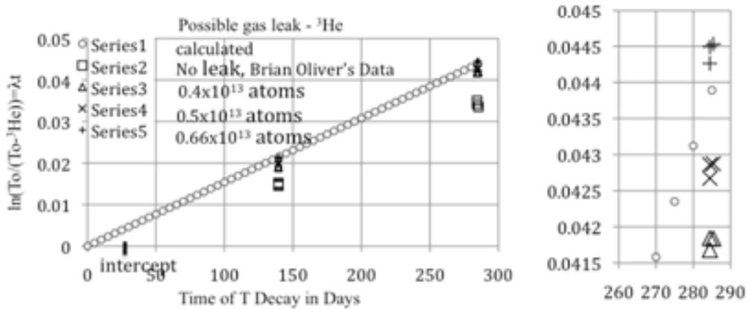
Fig. 4a,b - Graph of the MS data. Leak of gas during storage of 139 days (leaked atoms of <sup>3</sup>He corrects the data)
