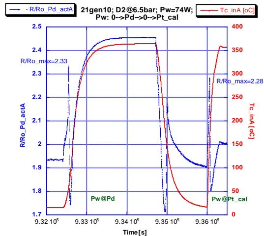
Fig.6. - R/Ro versus kind of power applied.
