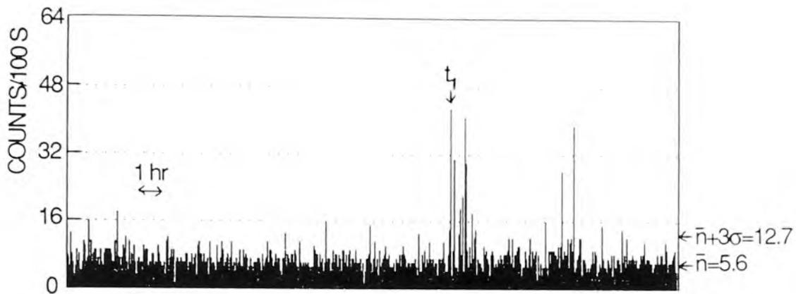
Fig.3(a) Neutron Bursts in Exp.II Measured with Sys.A(4-5 Feb.1991).
