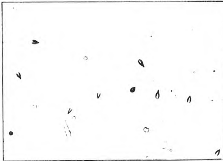
Fig.3 Tracks from American Palladium Foil
