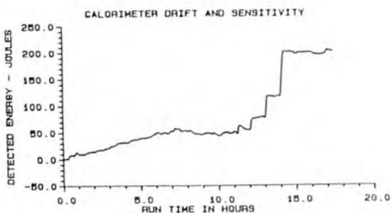
Figure 3. Calorimeter drift and sensitivity. The first ten hours show typical drift for the calorimeter operating at 8 watts total power. At hour 10 and at each hour following, calibration pulses of 5, 10, 20, 40, and 80 joules were inserted by a separate heater not in the computed energy balance.
