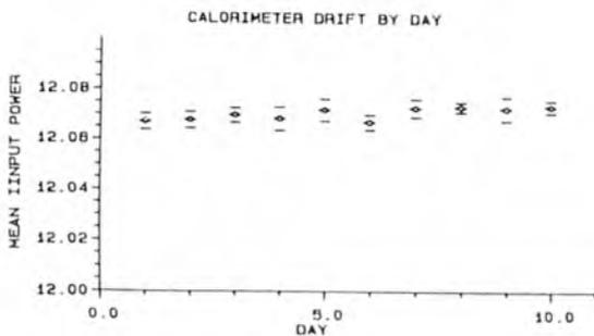
Figure 5. Calorimeter drift by day. The data of Figure 4. plotted by day. The error bars are one sigma.
