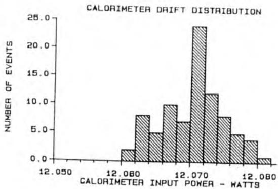
Figure 4. Calorimeter random drift test. In addition to the balance heater, the calorimeter is fitted with a heater driven by a random number generator. Every three hours the random value is changed. After two hours, the total power input is averaged over the third hour to determine a power value. The curve contains 86 three hour measurements, with a mean of 12.0784 watts and a sigma of 0.0044 watts.
