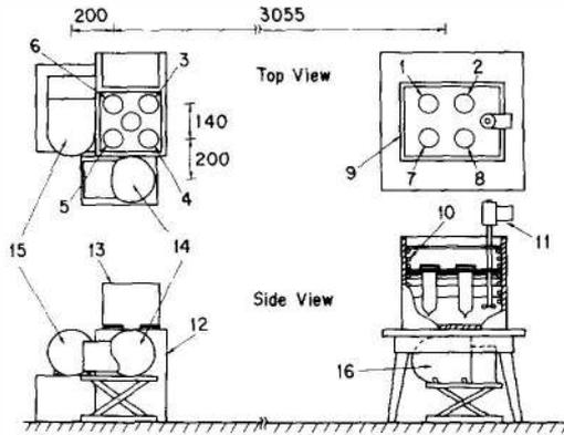
Figure 3. Setup of b) type experiment. 1 ~ 8 Dewar type cells in which 8 is for control experiment, 9 Coleman bath, 10 Cooling pipe, 11 Stirrer, 12 RTE220 bath, 13 Temperature controller, 14 <sup>3</sup>He rem-counter, 15, 16 BF<sub>3</sub> rem counters S/N 12254 and 9074, respectively.
