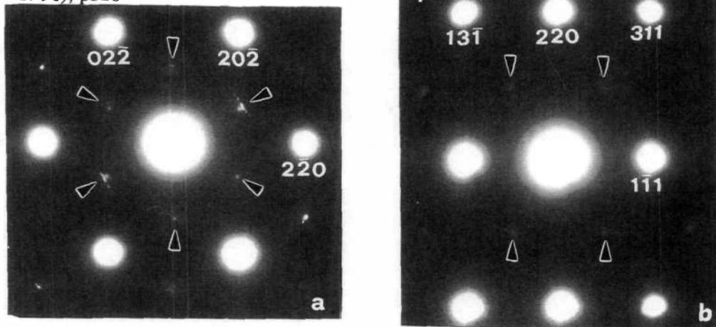
Figure 1. Experimental diffraction patterns of a) [111] zone axis and b) zone axis [112]
