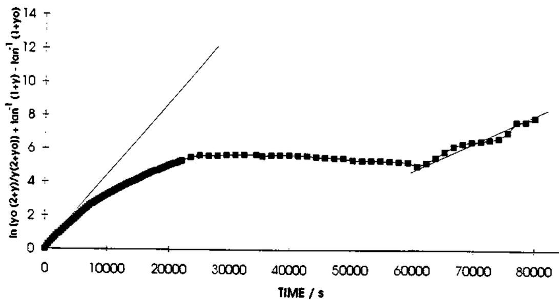
Fig 5. Analysis of a cooling curve according to equation (3) for an electrode following Scenario 4 - 1 mm diameter by 12.5 mm length Pd cathode polarised in 0.1M LiOD in D<sub>2</sub>O: final cell current: 250 mA; initial temperature for the cooling curve: 99.605°C.
