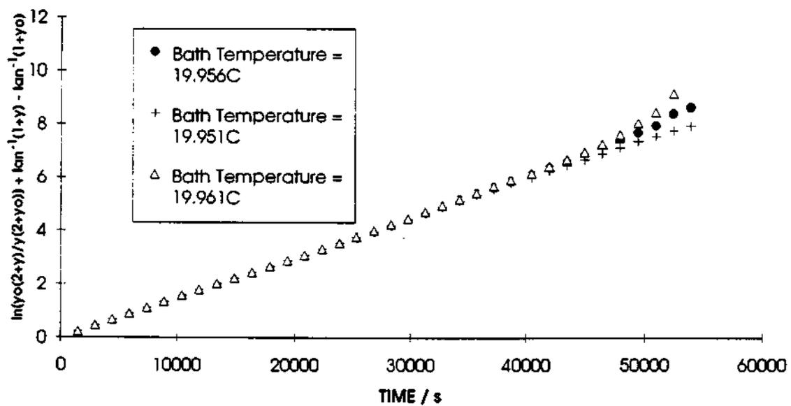
Fig 2. Analysis of a cooling curve according to equation (3) for an electrode following Scenario 2 - 1/4 mm diameter by 12.5 mm length Pd cathode polarised in 0.1M LiOD in D<sub>2</sub>O; final cell current: 200 mA; initial temperature for cooling curve: 51.524°C.
