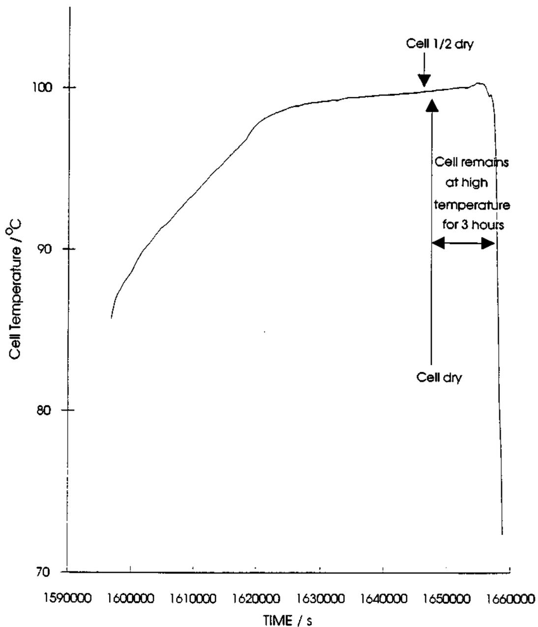
Fig 8. The temperature-time curve for a cell being driven to boiling showing also the initial part of the cooling curve - 2 mm length Pd cathode polarised in 0.1M LiOD in D<sub>2</sub>O; final cell current: 500 mA.
