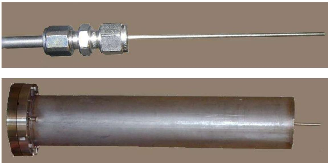
Figure 2. Top: photograph of the palladium tube. Bottom: photograph of the vacuum chamber.
