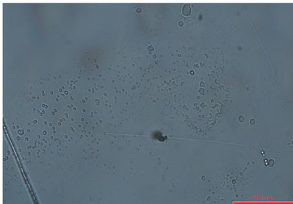
**Figure 12.** Track simulation with mechanical stress. The 200  $\mu\text{m}$  Pt wire is attached tightly to the surface of the Landauer CR-39 detector (scratch in the left corner of the image) for 2 days before etching. Etch time is  $t = 7.0$  hr. Lots of pits, mainly of small diameter ( $d < 4 \mu\text{m}$ ) are appeared. Compare the size of small pits with that seen in [663,435] image of Williams' detector.
