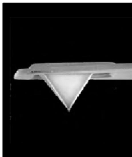
Fig. 2. SiN probe - side angle 35°, tip height 3  $\mu\text{m}$ .
