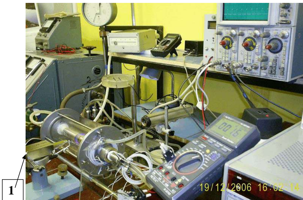
Figure 1. The gas glow discharge apparatus with CdTe detector.
