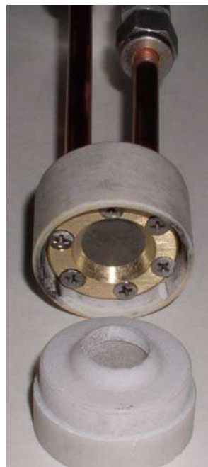
FIGURE 4. Exploded view of the cathode showing the insulating shroud. The cathode disc can be removed and is sealed using a rubber O-ring.
