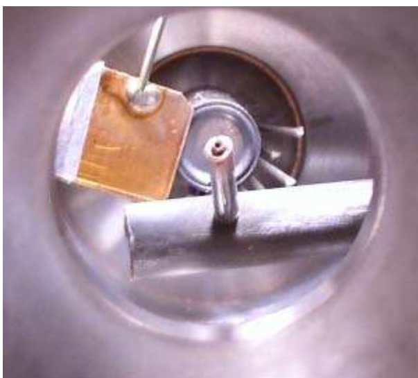
FIGURE 3. Cathode-eye view of the GM radiation detector. One of the copper absorbers is seen on the left. The anode is one of several designs using 2 mm wire covered by a glass insulator. The large tube from which it emerges is a glass-filled insulator.
