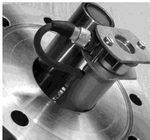
FIGURE 6. Si barrier detector (Ortec TB-016-050-1000) and GM tube ( 2.2\text{-}2.6\text{ mg/cm}^2 ).
