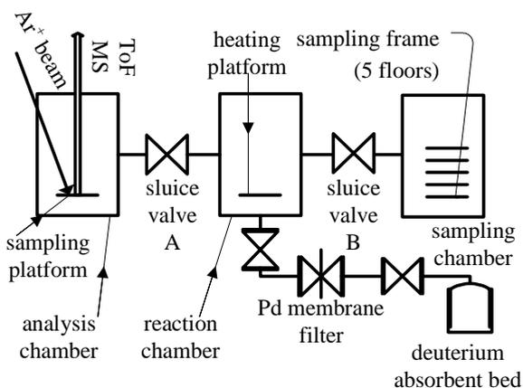
**Fig. 1. Schematic of purification and gas-solid reaction system.**
