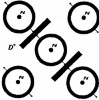
Fig. 2. The thin disks of the tetrahedral sites of the Pd lattice where the loading of deuterons takes place
