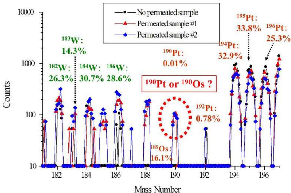
Figure 7. SIMS spectra for  $\text{D}_2$  permeated samples and no permeated sample.
