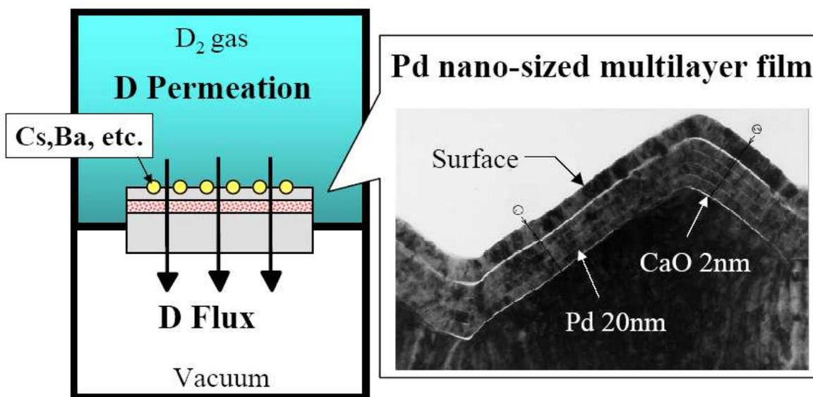
**Figure 1.** Experimental method for permeation-induced nuclear transmutation.
