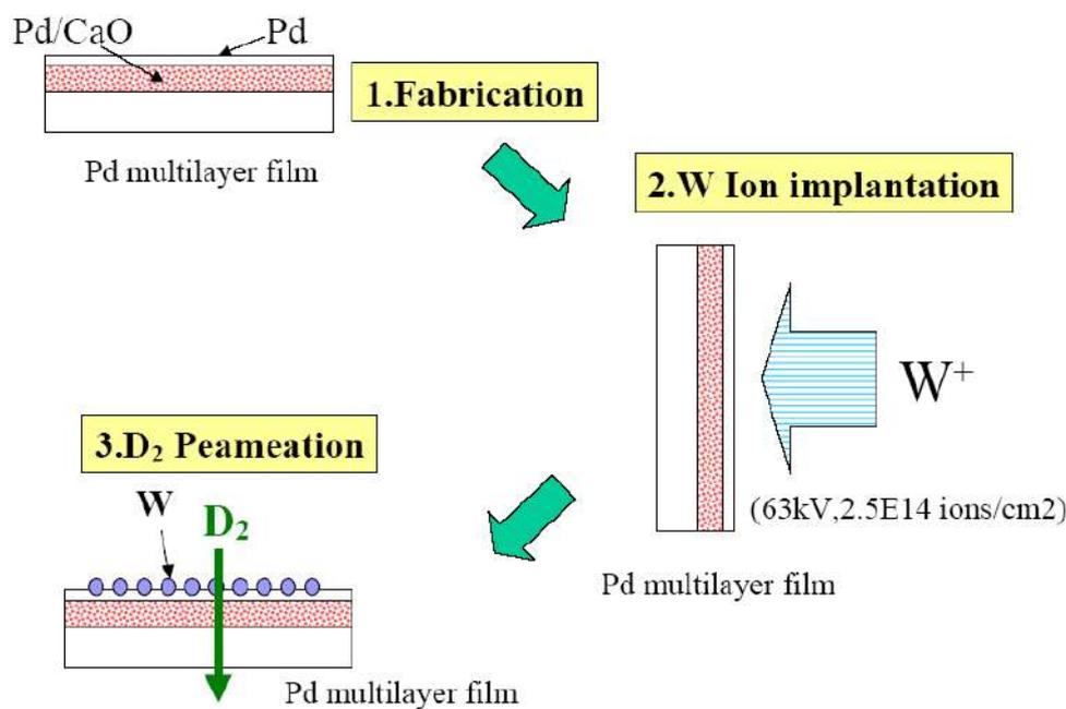
Figure 6. Experimental procedure of W transmutation experiment.
