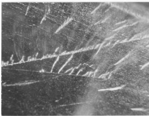
**Figure 4.** Bubbles of D<sub>2</sub> arising through acetone from cracks in PdD after electrolysis. The bright lines at which bubbles are forming are surface scratches that focused formation of a deeper crack structure.
