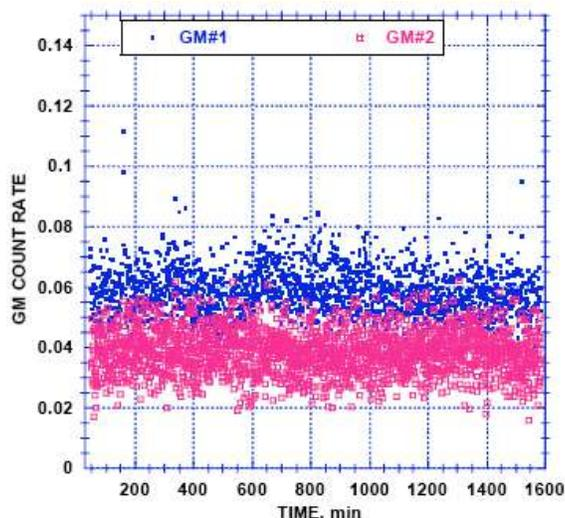
**Figure 19.** Behavior of GM No. 1 and GM No. 2 when a typical inert sample is in the apparatus. The difference between the two GM count rates is arbitrary. Only the constant value over time is important.
