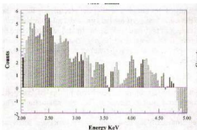
**Figure 3.** Count rate in excess of background for an active Ni cathode reported by Violante et al. [15].
