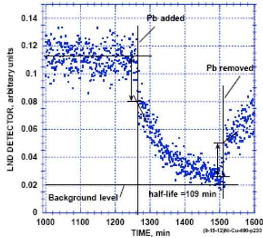
Figure 17. Effect of inserting a Pb absorber between 1262 and 1510 in shown in Fig. 16.
