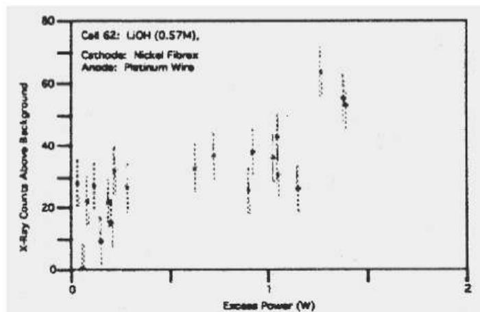
Figure 4. Radiation detected by Bush and Eagleton [17] from cell having a Ni cathode and H<sub>2</sub>O electrolyte while it was taking excess power.
