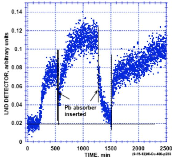
**Figure 16.** Behavior of radiation during the full study while Ni–Cu was being heated in H<sub>2</sub>.
