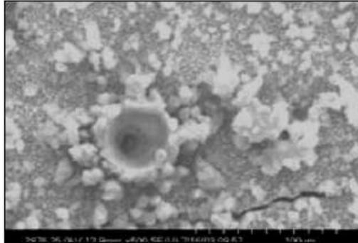
**Figure 1.** Large crater with a rounded shape. There are evident signs of melting of the ejected material, some of it solidified around the crater rim. The diameter is 50  $\mu\text{m}$ . The original point of the explosion seems to be located several tens of  $\mu\text{m}$  below the surface [3].
