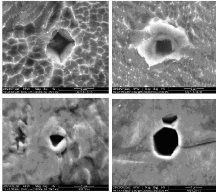
**Figure 4.** Micrographs of small craters from Super-wave experiments by M. Tsirlin . Published by Nagel [6]. The diameters range from 1μm to 2 μm. There are no signs of melting. The shapes appear to be influenced by the cathode crystal structure.
