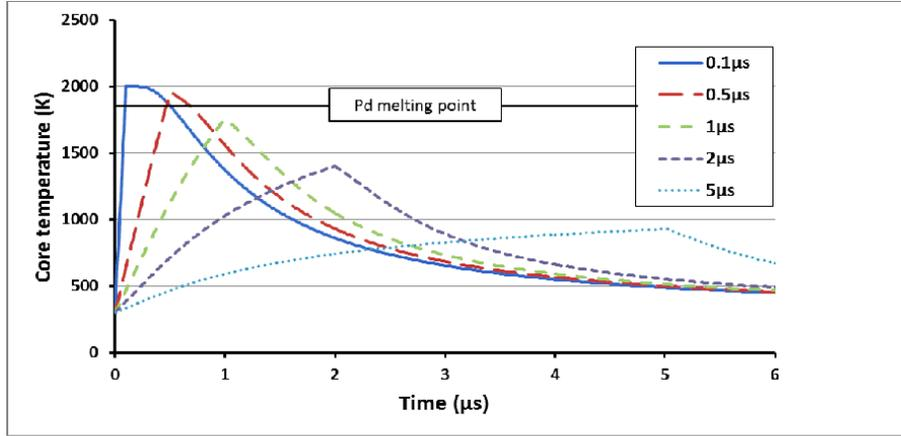
**Figure 12.** Evolution of the temperature at the centre of a 20  $\mu\text{m}$  core – Influence of the reaction time.
