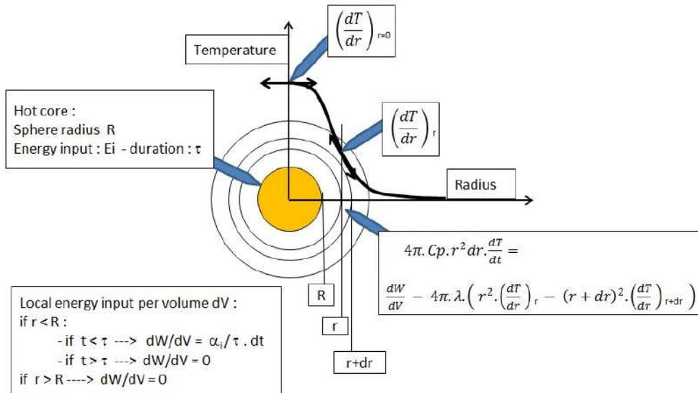
Figure 8. Schematic representation of the heat flow model.
