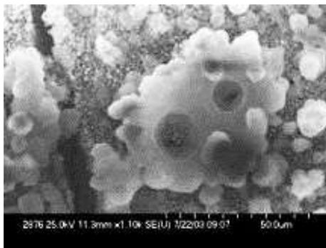
**Figure 2.** Two adjacent craters, 15 and 10  $\mu\text{m}$  in diameter. The larger one is fully rounded, while a hexagonal shape can still be recognized in the small one. Although both embedded within a common mass of molten material, they do not seem to be obviously correlated [3].
