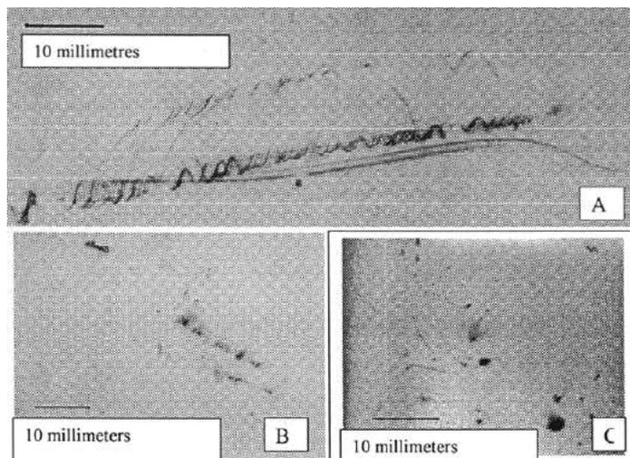
**Figure 14.** Markings on X-ray films set outside (A,B) and inside (C) vacuum chamber. Deuterium irradiation in glow discharge. The mark in A may record a spiral motion of an MBL or a revolution of two MBLs. The ones in B look like the ones Matsumoto called interference patterns. The ones in C look like ones Matsumoto photographed as well.
