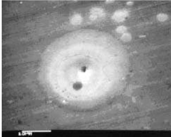
**Figure 1.** Entry pit of EV into aluminum sheet.
