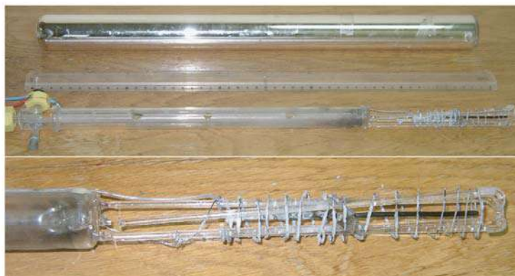
Figure 4. Top: a view of the Dewar. Bottom: views of the condenser and the cathode anode.
