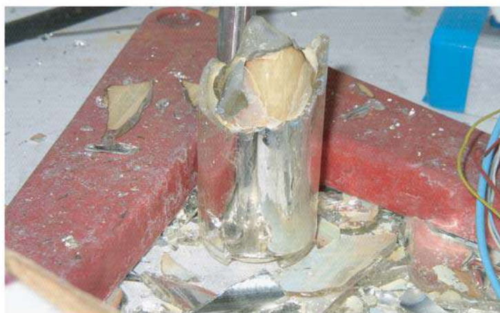
Figure 5. Remains of the Dewar cell after the explosion.
