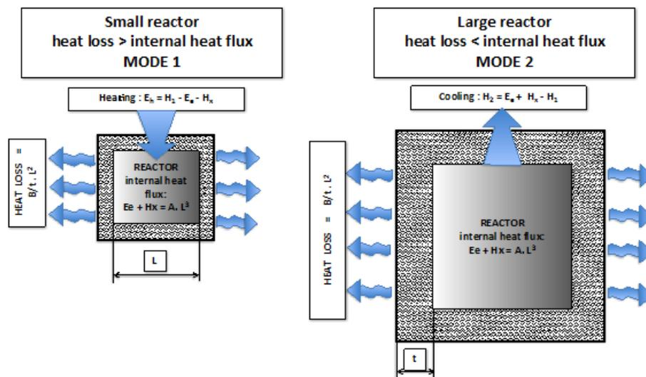
**Figure 8.** Influence of the reactor size – A larger unit may accommodate a thicker insulation – A given reactor technology operated in MODE 1 as a small unit may become a MODE 2 reactor in a larger size.
