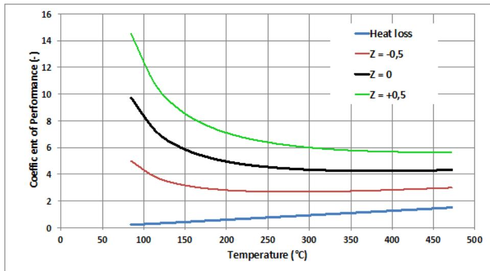
Figure 14. Relationship between the temperature and the COP for different  $Z$  values –  $\eta_m = 0.7 - f = 1 - T_{cold} = 25^{\circ}\text{C}$ .
