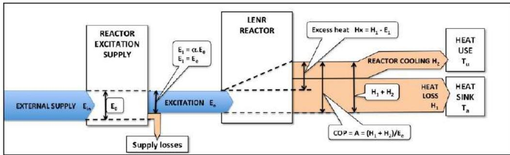
Figure 7. Energy flowchart for a cooled reactor (MODE 2).
