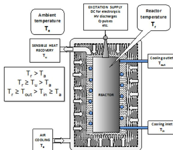
**Figure 9.** Active cooling. The thermal insulation is fitted with a laminar flow of gas that percolates inward. The gas leaves the enclosure at a temperature  $T_u$  that is higher than  $T_a$  and may be as high as  $T_r$ . The heat loss is recovered at a temperature above  $T_a$  and may have an usage.
