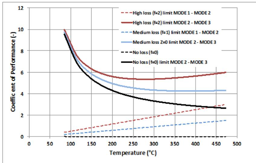
Figure 16. Limits of the different domains for several heat loss factors –  $\eta_m = 0.7 - T_{cold} = 50^\circ\text{C}$ .
