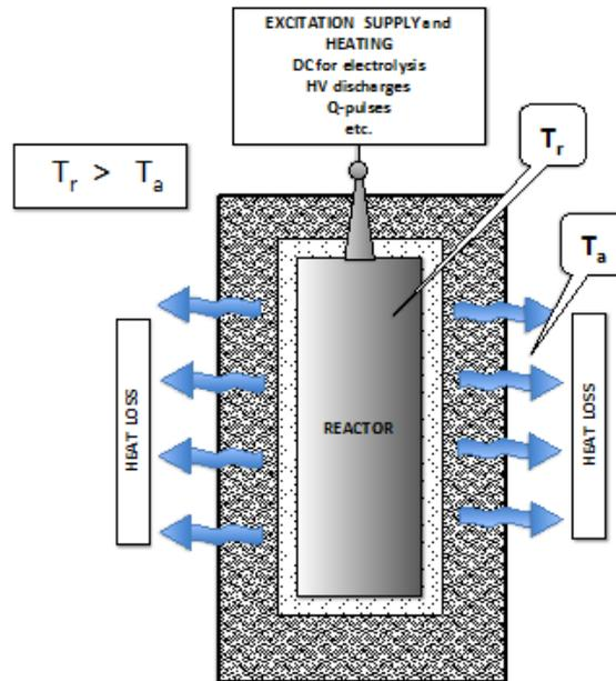
**Figure 2.** Schematic of a simple LENR reactor. (a) Here, the heat flux is merely lost into the environment. No use can be made of the heat in this configuration. (b) Note however the presence of the thermal insulation, a compulsory feature of the system if we want to detect that  $T_r > T_a$ .
