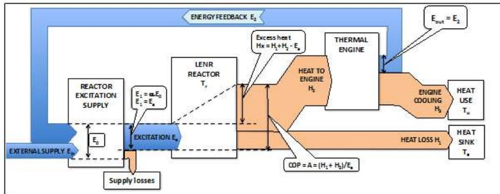
**Figure 10.** Mode 2 with feedback – The excess heat is transformed into electricity by a thermal engine coupled to a generator. This electrical energy  $E_{out}$  is fed back ( $E_2$ ) to the supply, reducing the external energy consumption.
