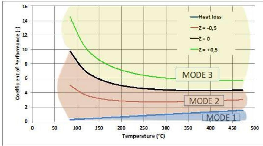
Figure 15. Operation mode domains as a function of the temperature and the COP –  $\eta_m = 0.7 - f = 1 - T_{cold} = 25^\circ\text{C}$ .
