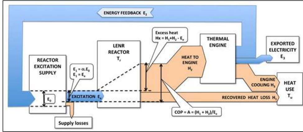
Figure 12. MODE 3 with recovery of the engine thermal output and active cooling.
