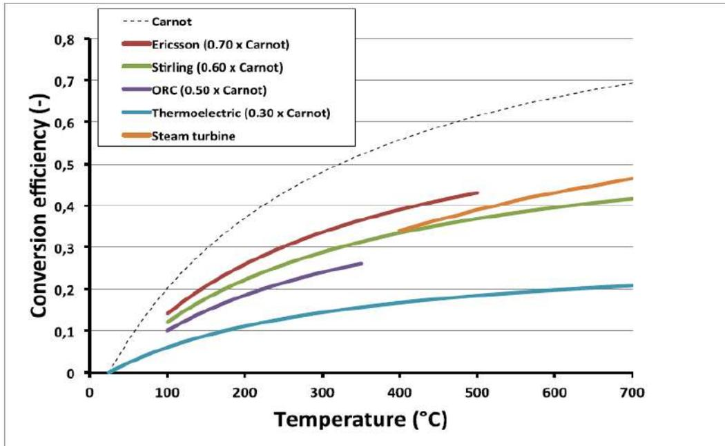
Figure 13. Relationship between the temperature of the heat source ( $T_{hot}$ ) and the typical efficiency of various thermal engines –  $T_{cold} = 25^{\circ}\text{C}$ .
