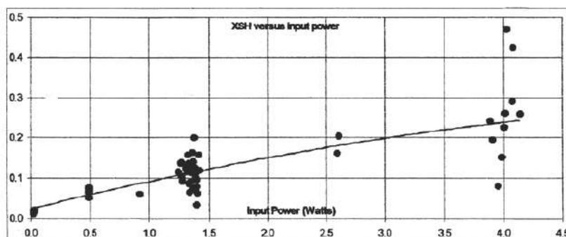
Figure 4. Excess heat (W) vs. input power (W).
