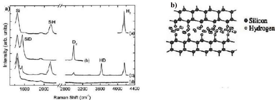
**Figure 7.** (a) Raman spectroscopy on Si surface implanted with hydrogen ions at 470 K showing the presence of H<sub>2</sub> molecules in nanometric cavities. From [31]. (b) Diagram of H<sub>2</sub> molecules trapped in Si nanometric cavities. From [29].
