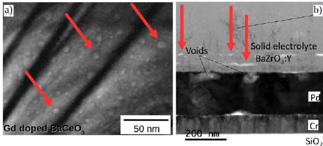
**Figure 10.** TEM images of nanometric cavities in polycrystalline proton conductors. Red arrows highlight some nanometric cavities. (a) Plane view in Gd-doped BaCeO<sub>3</sub> used below 770 K. From [41]. (b) Cross-section side view in Y-doped BaZrO<sub>3</sub> used at 590 K. From [42].
