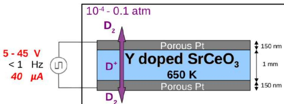
**Figure 1.** Mizuno's experimental system to study CMNS using a polycrystalline proton conductor based on Y-doped SrCeO<sub>3</sub> as solid electrolyte with D<sub>2</sub>. From [8].
