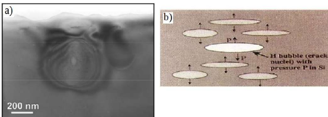
**Figure 8.** (a) Cross-section TEM image showing a nanometric cavity pressurized by its internal H<sub>2</sub>, and the long-range surrounding strain field, deep under the free surface of a hydrogenated Si wafer below 470 K. From [28]. (b) Diagram showing the pressure of H<sub>2</sub> in nanometric cavities on the Si crystalline matrix. From [29].
