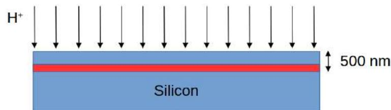
**Figure 4.** Ionic implantation of  $\text{H}^+$  in silicon crystals.
