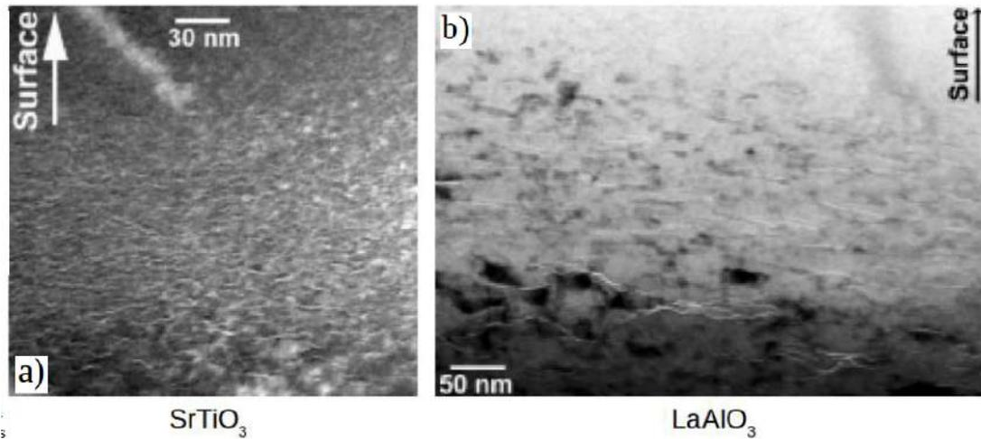
**Figure 9.** TEM images of high local densities of hydrogen related nanometric cavities (*side view*) in metal oxides with perovskite structure near their surfaces. These samples were implanted with hydrogen at 300 K for SrTiO<sub>3</sub> (a) and 570 K for LaAlO<sub>3</sub> (b). From [38].
