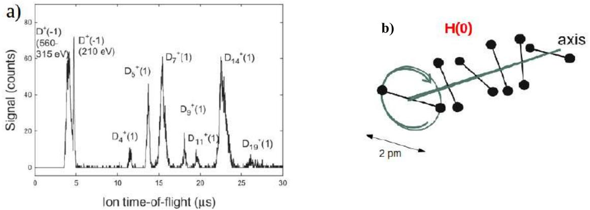
**Figure 3.** (a) Laser induced Coulomb explosions with time-of-flight mass spectroscopy near the surface of a metal oxide based on K-doped  $\text{Fe}_2\text{O}_3$ . The two first peaks correspond to closely spaced deuterons (2 pm). From [13]. (b) Hypothetical ultradense hydrogen Rydberg matter  $\text{H}(0)$ . From [18].
