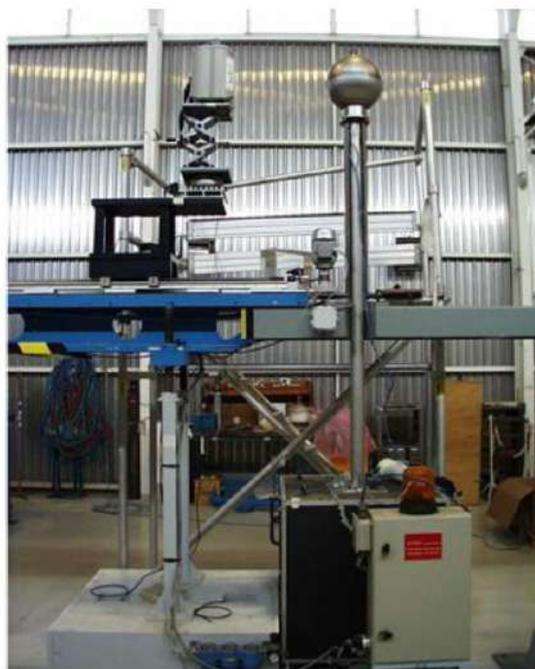
**Figure 2.** Experimental set-up showing a neutron dosimeter calibration. During the 18 April experiment, the neutron sources were located inside the black cubic container about 2 m from the electrolysis cell.
